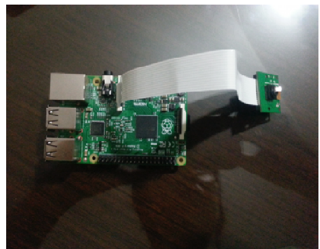
Fig. 5. Picamera attached to Raspberry Pi
